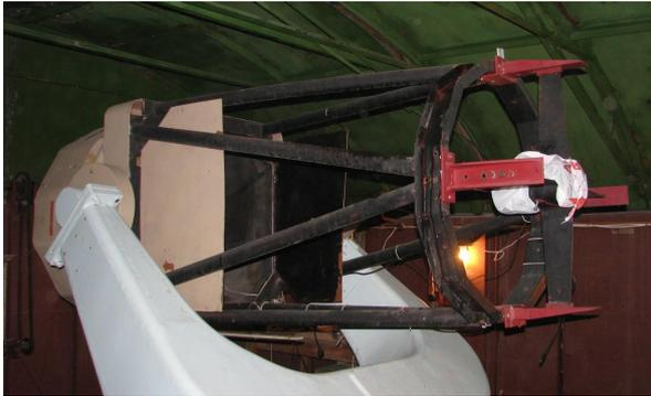
Fig. 2. Upgraded 80 cm telescope K-800 with field of view 55 minutes in Terskol, North Caucasus
